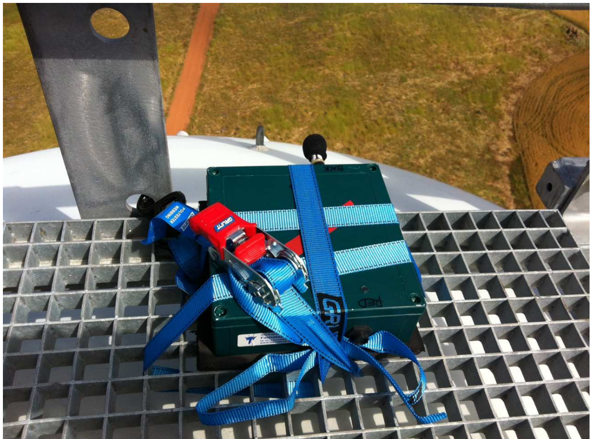
Plate 2. SM2 ultrasonic bat detector mounted on the galvanised mesh platform located on the nacelle of the Goldwind turbines.
