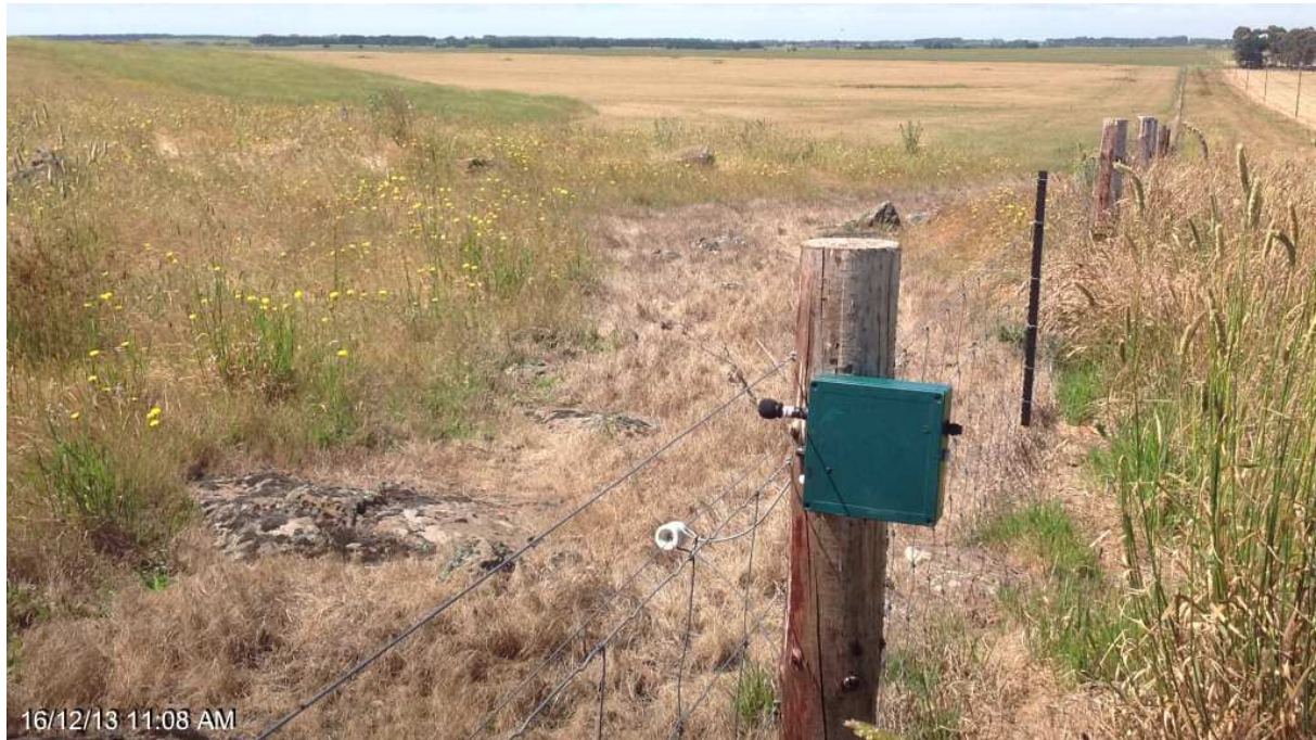
Plate 1. SM2 detector mounted on a fence post.
